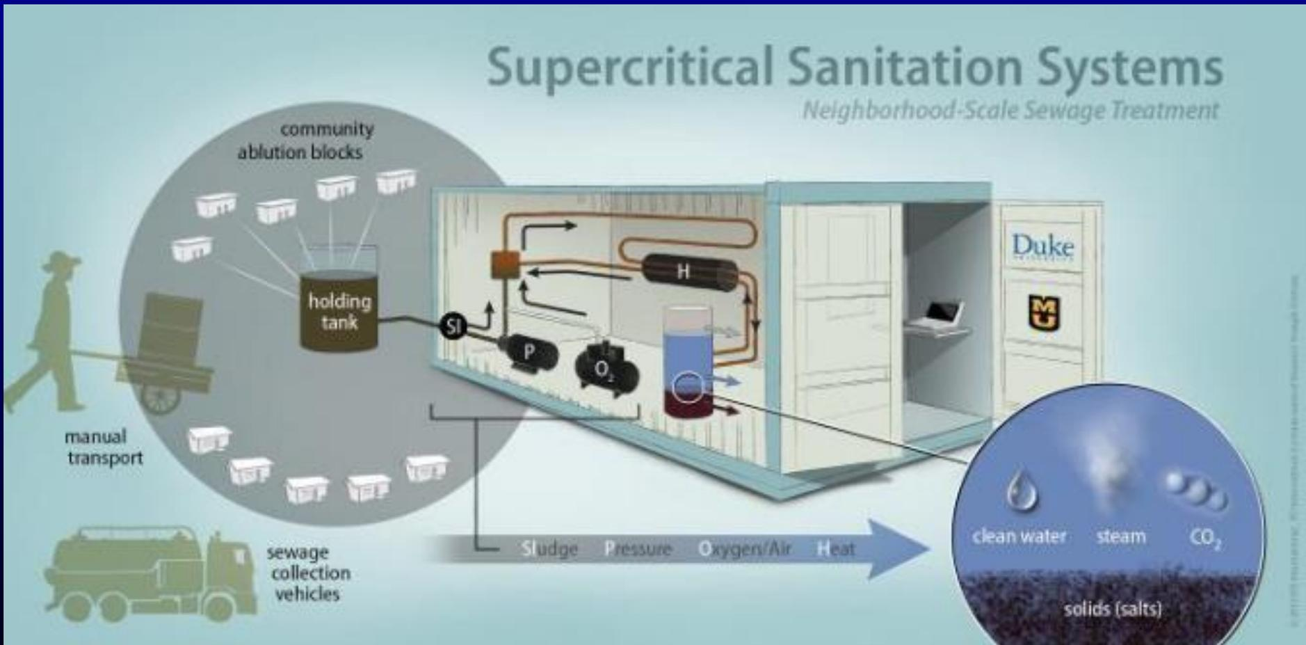
**In supercritical water, organics are rapidly oxidized (in seconds) resulting in heat, and CO<sub>2</sub>**
