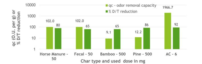
Figure 1: Odor removal from the ORS + 1 ppm H<sub>2</sub>S using AC and different biochars
