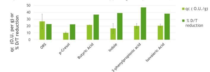
Figure 2: Odor removal using activated carbon (AC) for individual compounds and ORS at a 50 mg char dose
