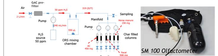
Fig. 3 - Dynamic adsorption schematics; picture of the portable olfactometer
