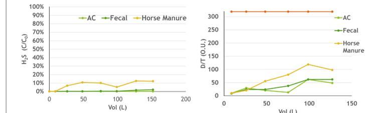
Fig. 4 - H<sub>2</sub>S breakthrough (left), and D/T breakthrough (right) as a function of air volume passed through the adsorption columns
