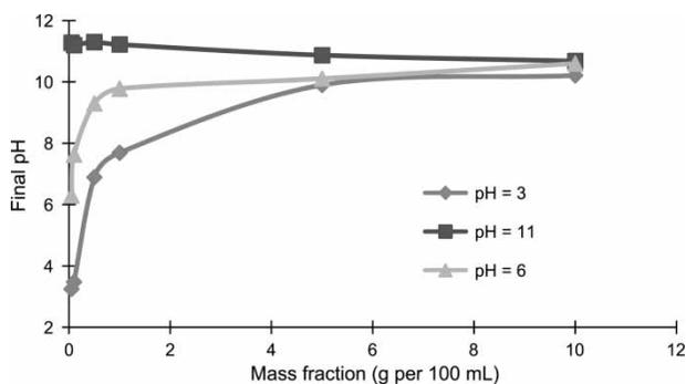
Figure 1. Point of zero charge determination. Final pH as a function of PAC mass fraction in the solution.
