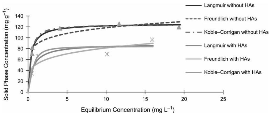
Figure 7. Adsorption isotherms for ketoprofen in the presence and absence of SRHAs using three widely used models.
