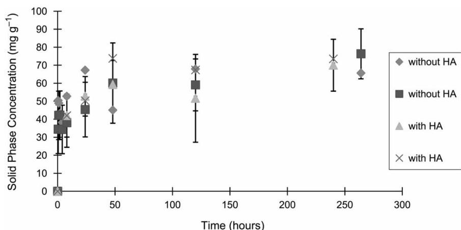
Figure 2. Adsorption kinetics of clofibric acid with and without humic acids in the solution. Error bars show one standard deviation from means. The different symbols are for two different experiments.
