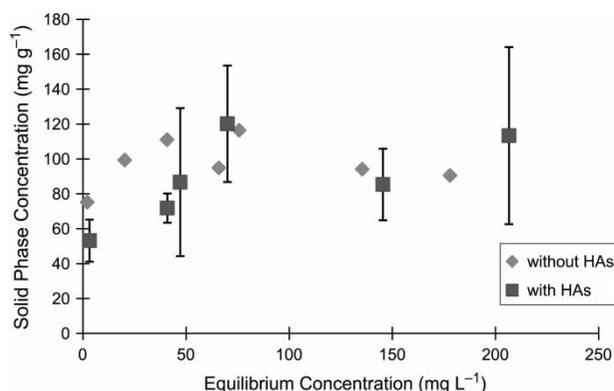
Figure 4. PAC adsorption capacity for clofibric acid in the presence and absence of humic acids. The error bars represent the standard error.
