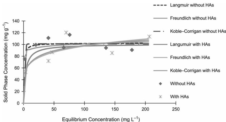
Figure 6. Adsorption isotherms for clofibric acid in absence of SRHAs using three widely used models.
