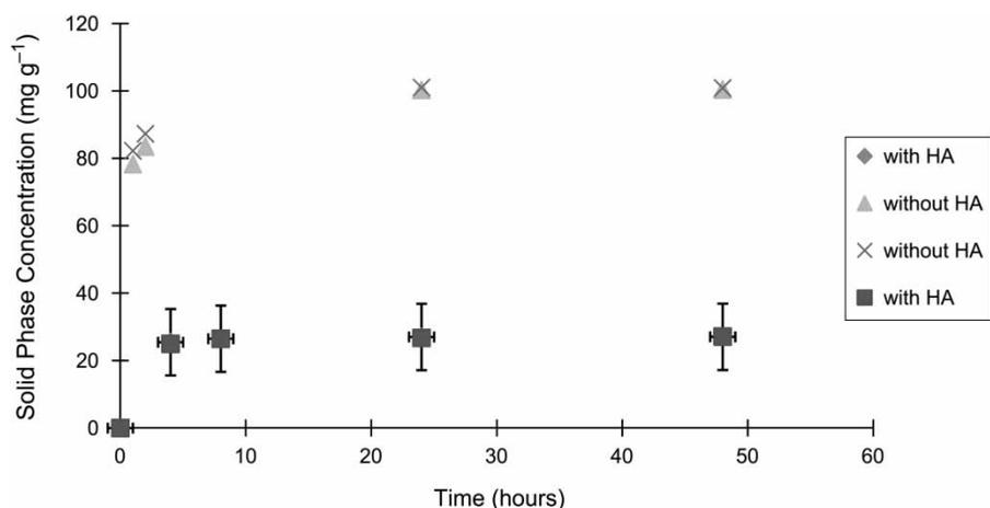
Figure 3. Adsorption kinetics of ketoprofen with and without humic acids in solution. Error bars show one standard deviation from means of one replicate. The different symbols are for two different experiments. Error bars or symbols that are not discernible are behind other symbols.
