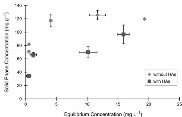
Figure 5. PAC adsorption capacity for ketoprofen in the presence and absence of humic acids. The error bars represent the standard error.
