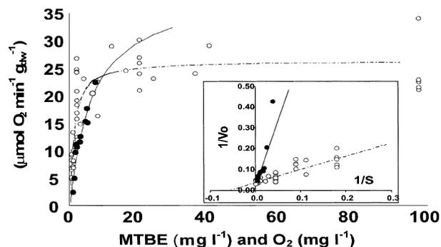
**Fig. 3.** Dissolved oxygen uptake rate of whole resting cells as a function of MTBE concentration (open circles) and as a function of dissolved oxygen concentration (closed circles). The inset shows the double reciprocal plot.
