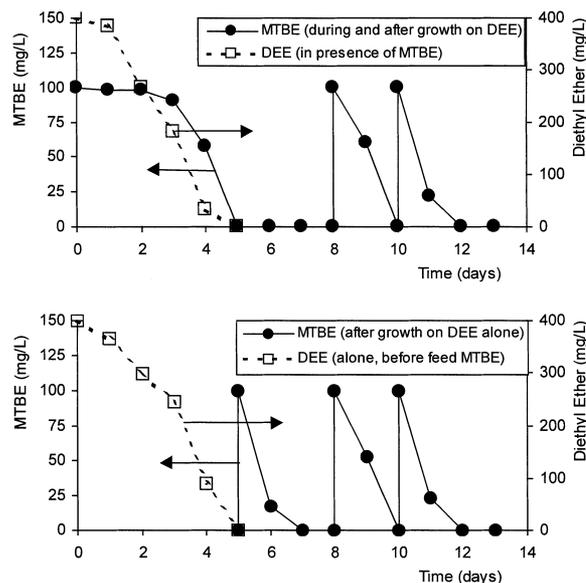
**Fig. 2.** MTBE biodegradation during and after growth on diethyl ether (DIEE) as an example of an alternative carbon source. Top graph: DIEE in the presence of MTBE before MTBE spikes on days 8 and 10. Bottom graph: DIEE alone before MTBE spikes on days 5, 8 and 10.
