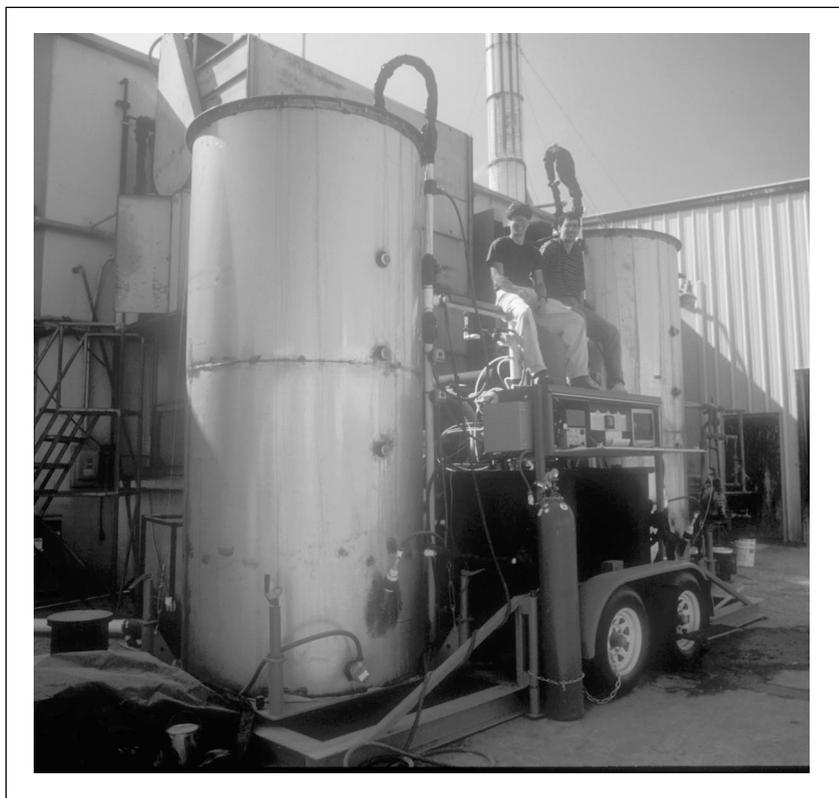
**Figure 3.** The constructed biotrickling filter.
