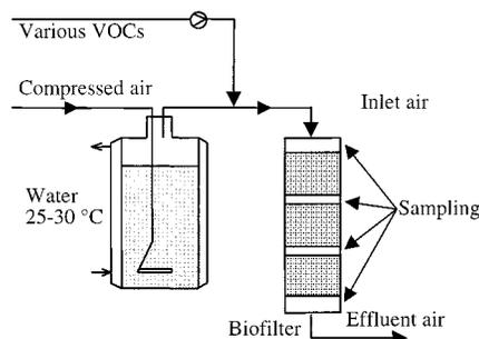
FIGURE 2. Schematic of the experimental setup.
