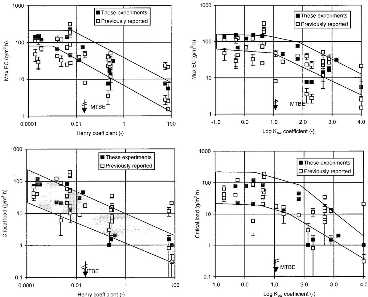
FIGURE 8. Experimentally determined and previously published maximum elimination capacities of the tested VOCs as a function of their dimensionless Henry and logarithm of octanol/water partition coefficients. All values of Table 2 are reported. Henry and octanol/water partition coefficients were obtained from refs 46–51. The gray area represents the general trend.
