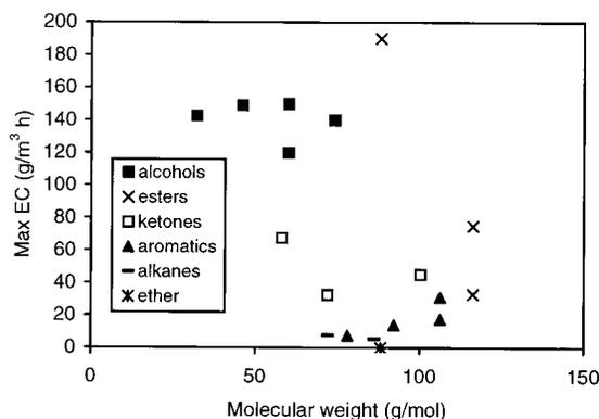
**FIGURE 7. Average of experimentally determined maximum elimination capacities of VOCs by classes of compounds and molecular weight.**
