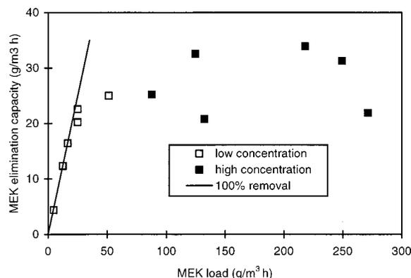
**FIGURE 5.** Typical results of the test protocol: MEK elimination capacity as a function of the loading.
