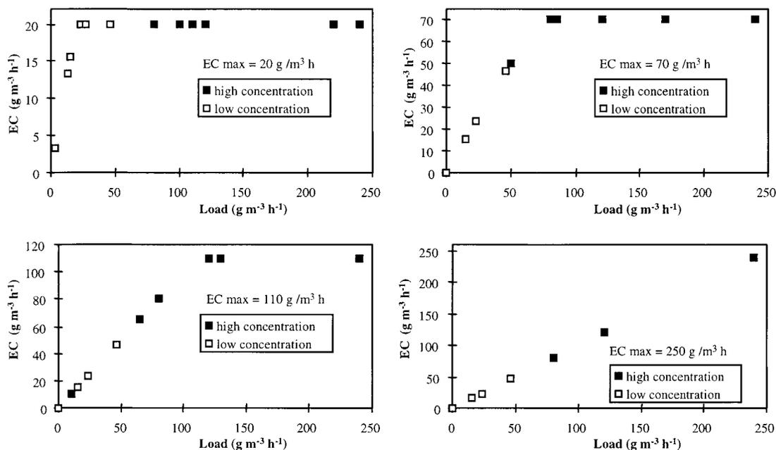
FIGURE 3. Computed elimination capacity vs pollutant load plots for the proposed protocol assuming simple kinetics (see text for details) for four different maximum elimination capacities. Conditions: air flow rate of  $1 \text{ m}^3 \text{ h}^{-1}$  (surface loading of  $55 \text{ m}^3 \text{ m}^{-2} \text{ h}^{-1}$ ); inlet pollutant concentration of  $0.35 \text{ g m}^{-3}$  (open symbols) and  $1.8 \text{ g m}^{-3}$  (closed symbols).
