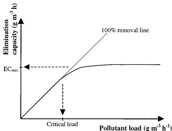
FIGURE 1. Typical elimination capacity vs load characteristic in a biofilter.  $EC_{max}$  is the maximum elimination capacity; the critical load is the maximum loading at which the removal efficiency starts to deviate significantly from the 100% removal line.
