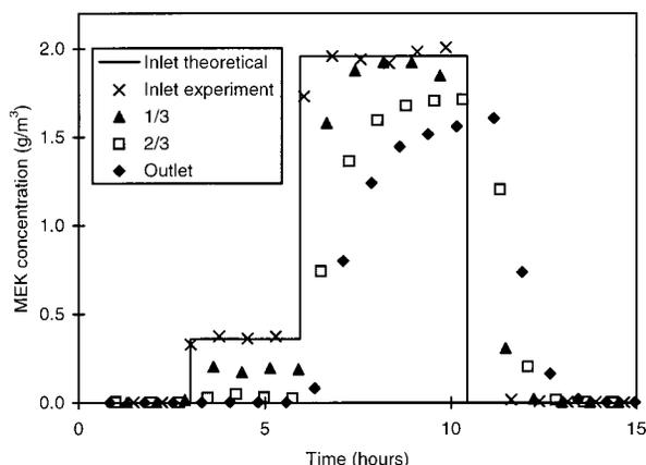
**FIGURE 4.** Typical results of the test protocol (MEK shown): concentrations of MEK at different heights in the biofilter vs time.
