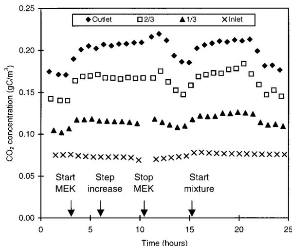
**FIGURE 6.** Typical results of the test protocol: concentrations of CO<sub>2</sub> at different heights in the biofilter vs time during the MEK run. Note the extended scale.
