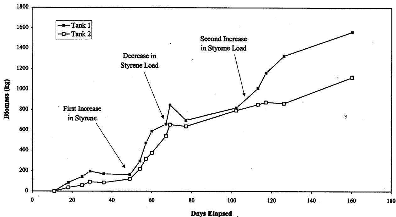
FIGURE 5. Biomass accumulation after styrene load additions to the system. Secondary load increase not discussed in paper.
