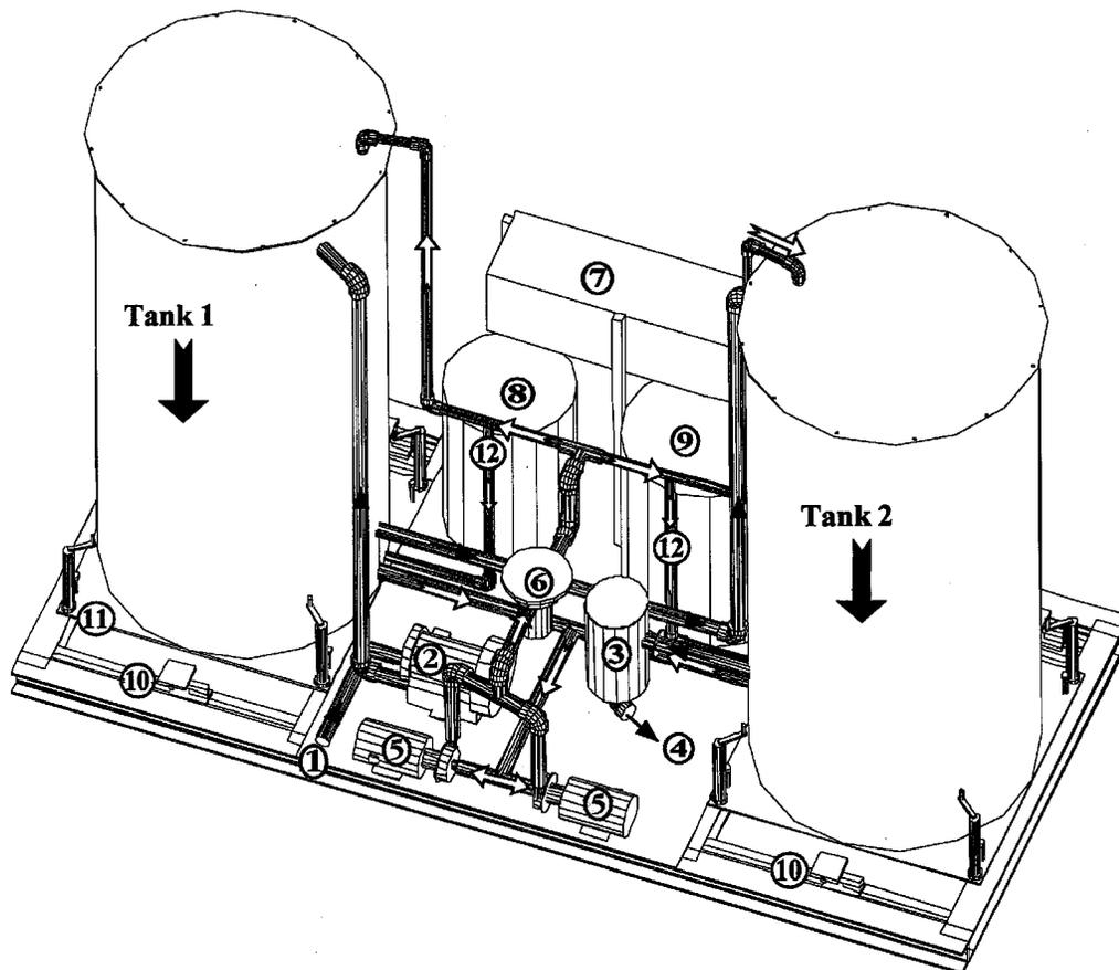
FIGURE 2. Design drawing of the pilot-scale biotrickling filter reactor. Open arrows: water flow; filled arrows: air flow. (1) contaminated inlet air; (2) blower; (3) knock-out pod; (4) purified outlet air; (5) water pumps; (6) strainer basket; (7) computer control box; (8) nutrient tank; (9) caustic tank; (10) sliding load cells (outside position); (11) jacks; (12) water return to tank bottoms (for mixing).
