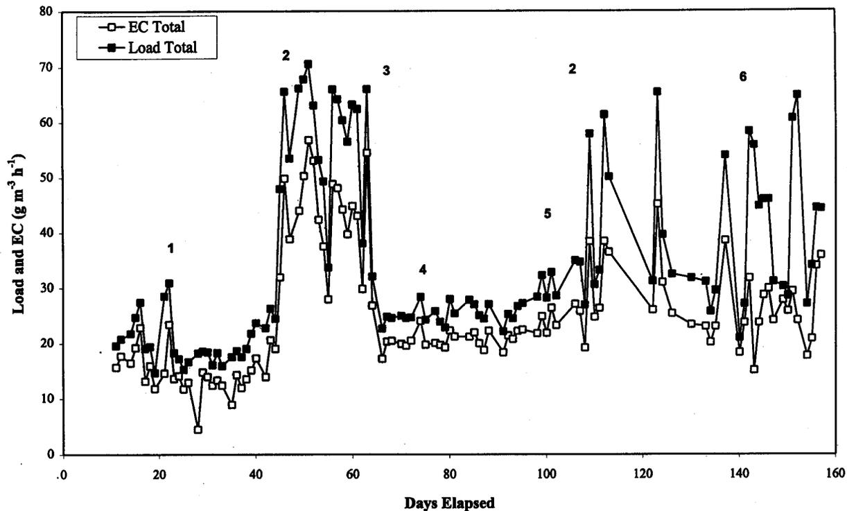
FIGURE 4. Total load and elimination capacity for biotrickling filtration system. System experiments occurred: (1) nutrient concentration in water doubled; (2) styrene load artificially increased; (3) artificial styrene load decreased; (4) heating element turned off; (5) tracer test performed; (6) microbiological substrate uptake rate study performed.
