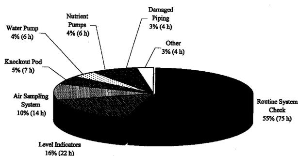
FIGURE 3. The distribution of time (% and hours) required for routine system checks and maintenance on different malfunctioning systems over a five-month operating period. Total hours = 138 h.
