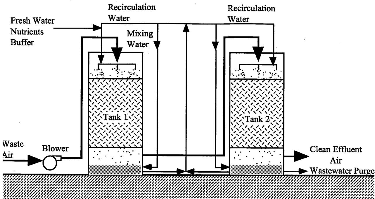
FIGURE 1. Schematic of the biotrickling filter system. For this cocurrent system, air is passed through the two tanks in series and water is applied in parallel.
