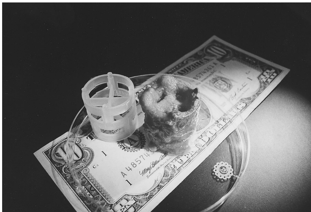
Fig. 2. Picture of a clean Pall ring (left) and one covered with biomass (right) before cleaning. Since the biomass content was very high, a large portion of the inner volume of the ring was filled with biomass.
